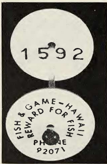
FIG. 20. Petersen disk tag used in tagging Acanthurus triostegus sandvicensis on Oahu. The ends of the monofilament nylon connecting the disks have been melted into knobs with a cigarette lighter. The heating caused a blackening of the one knob which is visible.
